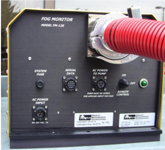
Figure 2: Fog Monitor Control Panel
