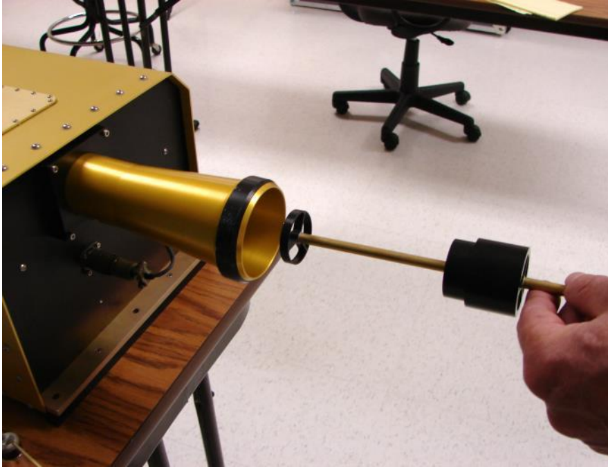
Figure 29: Inserting the Calibration Fixture into the Fog Monitor. The calibration fixture should be placed as far into the instrument's inlet as it will comfortably go.
