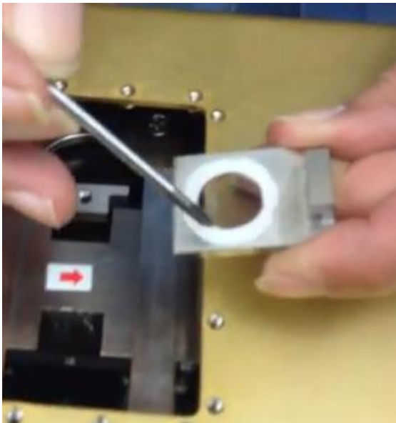
Figure 17: Removed Window with O-Ring
