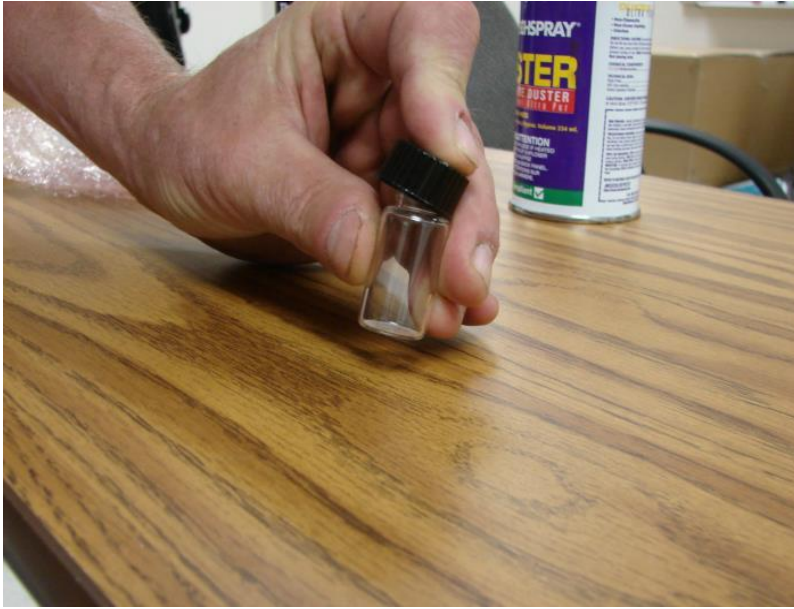
Figure 27: Tapping the Bead Dispenser to Dislodge Beads
