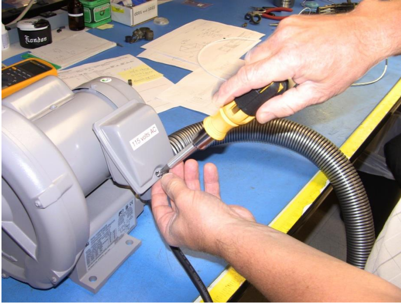
Figure 3: Unscrewing Pump Lid
